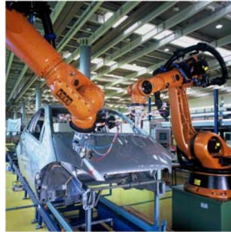
Fully automated marking of paint defects (Car Paint Vision)
