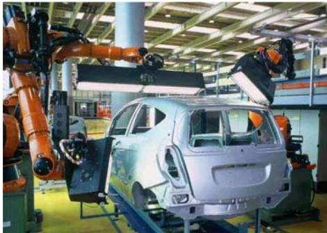
Paint inspection of complete car bodies (Car Paint Vision)
